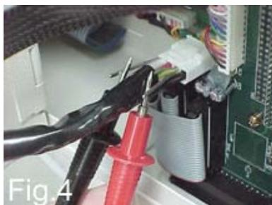
Now carefully apply the red test lead to the needle for the white wire and the black lead to the needle for the green wire (fig.4). Allow the meter a few seconds to adjust and then read the display (fig.5). For normal operation, you should have a reading of **5.03 to 5.08** volts. If your reading is within this range, there is no need to adjust the 5 volt power
