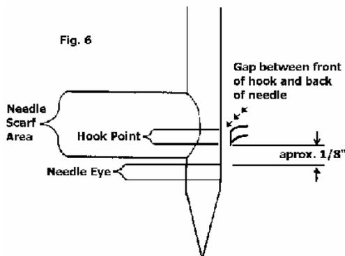
12. Firmly tighten the screw on the bottom right side of the hook. Then, rotating the degree wheel, tighten the other two screws of the hook.
