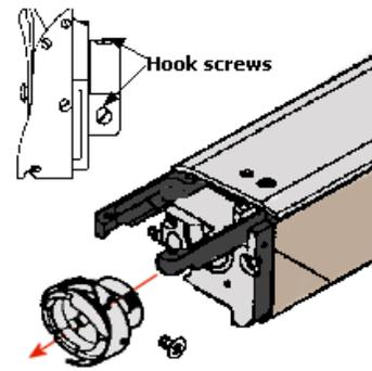
7. Remove the hook from the lower shaft of the machine and inspect it:
